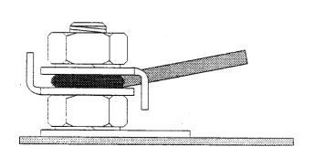
Ensure that the incoming supply wires are connected to the input bolts as shown and that the NUTS ARE SECURELY TIGHTENED.
